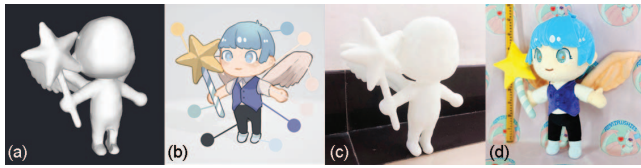
Figure 11: We use 3DBrushVR to design the toy. (a)The modeling result. (b)The color design draft. (c)The 3D print results. (d)The plush toy.
