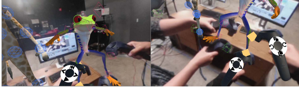
Figure 1: A pair of simultaneously captured images from the first-person view of each user within the dyad in mixed reality environment. Each user can cooperate to adjust the pose of the shared character naturally in 3D using inverse kinematics. Left: posing the left leg of the frog. Right: posing the right leg of the frog.
