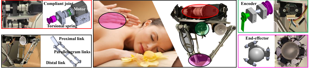
Figure 1. The design of the proposed parallel massage manipulator consisting of compliant joints, encoders, links and end-effector. A potential application scenario where the proposed massage robot can perform a tapping massage task (Middle figure).
